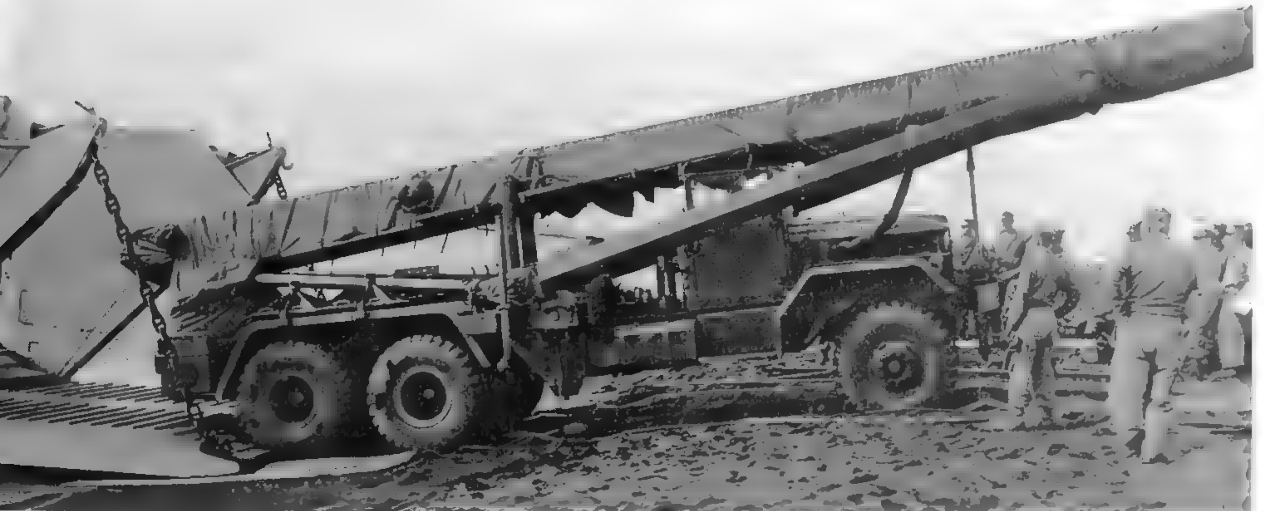
The M139C chassis, used by the M289, had a reduced normal axle ratio to permit reasonable off-road maneuverability, despite the heavy load. The M289 leaving this landing craft has been prepared for deep-water fording. (Photo courtesy of United States Army Engineer School History Office)
